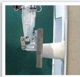
制品臂轻微接触纸杯时感应干涉，动作停止 The product arm slightly resists the paper cup when the induction interference, the movement stops
