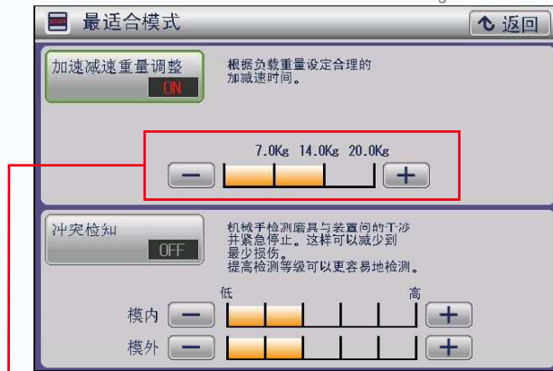
输入夹具和产品的重量 Enter the weight of chuck and product
