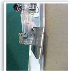
制品臂压瘪一次性纸杯，撞上固定支架 The product arm flattens the disposable paper cup and hits the fixed bracket
